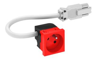
Ready-for-connection protective contact socket Single  $33^{\circ}$ , with increased touch protection, incl. 0.25 m connection cable with GST18 connector and locking clip, 16 A, 250 V~.
