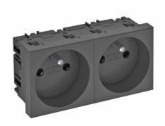
Socket with earthing pin, double  $0^\circ,$  with increased touch protection, with screwless terminals, 2-pin, 16 A, 250 V~, with connection terminals to IEC 60884-1.
