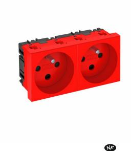
Socket with earthing pin, double 0°, encoded version, with increased touch protection, with screwless terminals, 2-pin, 16 A, 250 V~, with connection terminals according to IEC 60884-1.
