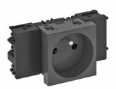
Earthing pin socket with connection to side, Single 0°, with increased touch protection, with screwless terminals, 2-pin, 16 A, 250 V $\sim$ , with connection terminals to IEC 60884-1, suitable for the installation in Rapid 45 device installation trunking systems.
