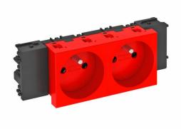
Earthing pin socket with connection to side, Double  $0^\circ$ , with increased touch protection, with screwless terminals, 2-pin, 16 A, 250 V~, with connection terminals to IEC 60884-1, suitable for the installation in Rapid 45 device installation trunking systems.
