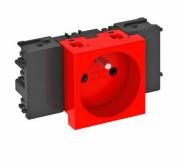
Earthing pin socket with connection to side, Single 0°, with increased touch protection, with screwless terminals, 2-pin, 16 A, 250 V $\sim$ , with connection terminals to IEC 60884-1, suitable for the installation in Rapid 45 device installation trunking systems.
