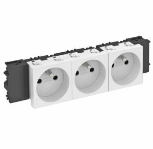
Earthing pin socket with connection to side, Triple 0°, with increased touch protection, with screwless terminals, 2-pin, 16 A, 250 V~, with connection terminals to IEC 60884-1, suitable for the installation in Rapid 45 device installation trunking systems.
