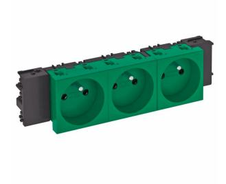
Earthing pin socket with connection to side, Triple  $0^\circ$ , with increased touch protection, with screwless terminals, 2-pin, 16 A, 250 V~, with connection terminals to IEC 60884-1, suitable for the installation in Rapid 45 device installation trunking systems.
