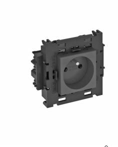
Earthing pin socket with connection to side, Single 0°, with increased touch protection, with screwless terminals, 2-pin, 16 A, 250 V~, with connection terminals to IEC 60884-1, suitable for the installation in Rapid 80 device installation trunking systems.
