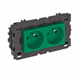
Socket with earthing pin with side connection Double 0°, with increased touch protection with screwless terminals, 2-pin, 16 A, 250 V~, with connection terminals to IEC 60884-1, suitable for installation in Rapid 80 device installation trunking systems.
