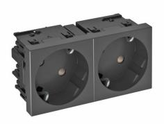
Protective contact socket double 33°, with increased touch protection, with screwless terminals, 2-pin, 16 A, 250 V $\sim$ , with connection terminals to IEC 60884-1
