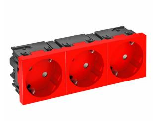
Protective contact socket triple 33°, with increased touch protection, with screwless terminals, 2-pin, 16 A, 250 V~, with connection terminals to IEC 60884-1.
