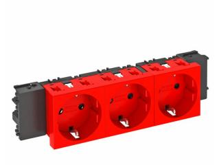
Protective contact socket with connection to side, triple 0°, with increased touch protection, with screwless terminals, 2-pin, 16 A, 250 V~, with connection terminals to IEC 60884-1, suitable for the installation in Rapid 45 device installation trunking systems.
