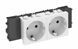
Protective contact socket with connection to side, Double 0°, with increased touch protection, with screwless terminals, 2-pin, 16 A, 250 V $\sim$ , with connection terminals to IEC 60884-1, suitable for the installation in Rapid 45 device installation trunking systems.
