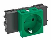
Protective contact socket with connection to side, Single 0°, with increased touch protection, with screwless terminals, 2-pin, 16 A, 250 V~, with connection terminals to IEC 60884-1, suitable for the installation in Rapid 45 device installation trunking system.
