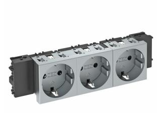
Protective contact socket with connection to side, triple 0°, with increased touch protection, with screwless terminals, 2-pin, 16 A, 250 V~, with connection terminals to IEC 60884-1, suitable for the installation in Rapid 45 device installation trunking systems.
