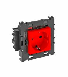
Protective contact socket with connection to side, Single 0°, with increased touch protection, with screwless terminals, 2-pin, 16 A, 250 V~, with connection terminals to IEC 60884-1, suitable for the installation in Rapid 80 device installation trunking system.
