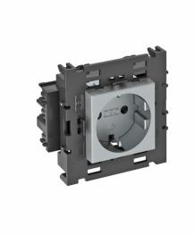
Protective contact socket with connection to side, Single 0°, with increased touch protection, with screwless terminals, 2-pin, 16 A, 250 V~, with connection terminals to IEC 60884-1, suitable for the installation in Rapid 80 device installation trunking system.
