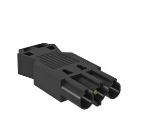
Connector part, 3-pin, type GST18i with screw connection, low height (no slot loss in combination with distributor blocks), for cross-sections of 0.75–2.5 mm<sup>2</sup>, single- and fine-wire cables connectable without end sleeve, for cable diameters between 6.5–10.5 mm (H05VV, NYM), unmounted with strain relief, terminable in situ, 250 V, 16 A.
