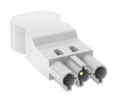
Connector part, 3-pin, type GST18i with screw connection for cables of 1.5–4.0  $\,$  mm² and cable diameters between 10.5–14.5 mm (H05VV, NYM), unmounted with strain relief, terminable in situ, 250 V, 16 A.
