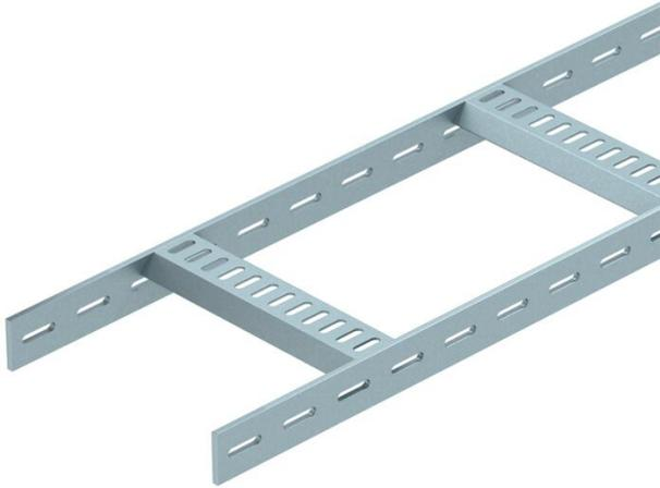
Shipbuilding cable ladder with perforated side rail of side height 40 mm with welded, perforated trapezoidal rungs which open in a downwards direction. Load tested according to IEC in conjunction with connector, type SLV. The shipbuilding cable ladder, including fittings, is also available in stainless steel on request. Powder coating according to RAL colours possible.
