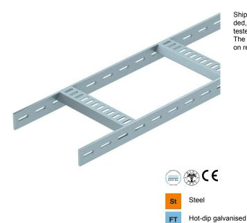
Shipbuilding cable ladder with perforated side rail of side height 40 mm with welded, perforated trapezoidal rungs which open in a downwards direction. Load tested according to IEC in conjunction with connector, type SLV. The shipbuilding cable ladder, including fittings, is also available in stainless steel on request. Powder coating according to RAL colours possible.
