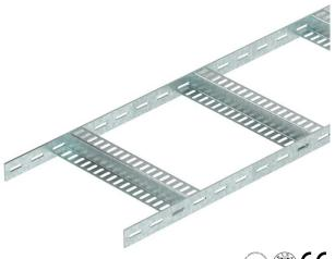
Light-duty shipbuilding cable ladder with perforated side rail of side height 35 mm with welded, perforated Z rungs. Load tested according to IEC in conjunction with connector, type SLV.
