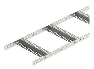
Light-duty shipbuilding cable ladder with perforated side rail of side height 35 mm with welded, perforated Z rungs. Load tested according to IEC in conjunction with connector, type SLV.
