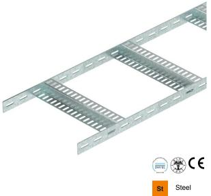
Light-duty shipbuilding cable ladder with perforated side rail of side height 35 mm with welded, perforated Z rungs. Load tested according to IEC in conjunction with connector, type SLV.
