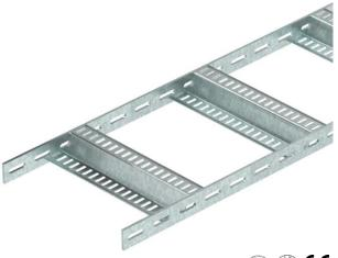
Shipbuilding cable ladder with perforated side rail of side height 40 mm with welded, perforated Z rungs. Load tested according to IEC in conjunction with connector, type SLV.
