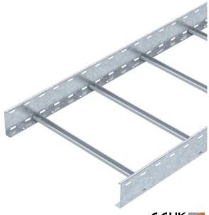
Cable ladder with 110 mm side height with welded C30 profile rungs which are open in an upwards direction. Rolled side rail for reinforcement and as edge protection. Fastening to the bracket takes place using clamps, type LKS 40. The slot dimension of the frame is 16.5 mm and the appropriate U clamp clip is type
