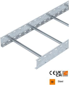
Cable ladder with 110 mm side height with welded C30 profile rungs which are open in an upwards direction. Rolled side rail for reinforcement and as edge protection. Fastening to the bracket takes place using clamps, type LKS 40. The slot dimension of the frame is 16.5 mm and the appropriate U clamp clip is type 2056.
