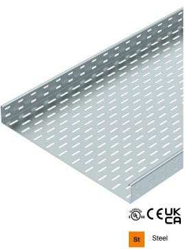
SKS 60 = heavy-duty cable tray system with 60 mm side height. The cable tray, type SKS, should also be used for the maintenance of electrical function. For additional data, please refer to BSS fire protection systems. Magnetic shield insulation without cover 20 dB, with cover 50 dB.
