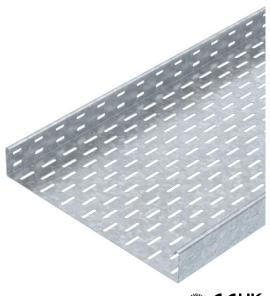
SKS 60 = Heavy-duty cable tray system with 60 mm side height. The cable tray, type SKS, should also be used for the maintenance of electrical function. For additional data, please refer to BSS fire protection systems. Magnetic shield insulation without cover 20 dB, with cover 50 dB.
