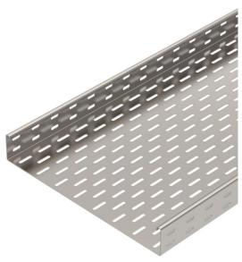
SKS 60 = Heavy-duty cable tray system with 60 mm side height. The cable tray, type SKS, should also be used for maintenance of electrical function. For additional data, please refer to BSS fire protection systems. The cable tray is fastened to the bracket with bolts, type FRS M6 x 12. Magnetic shield insulation without cover 20 dB, with cover 50 dB.
