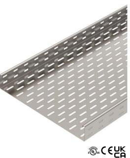
SKS 60 = heavy-duty cable tray system with 60 mm side height. The cable tray, type SKS, should also be used for maintenance of electrical func-tion. For additional data, please refer to BSS fire protection systems. The cable tray is fastened to the bracket with bolts, type FRS M6 x 12.
