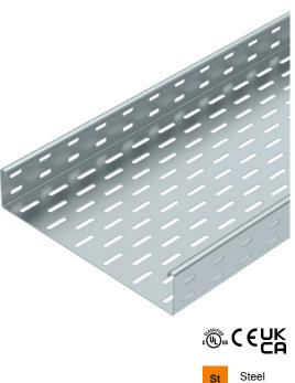
SKS 60 = heavy-duty cable tray system with 60 mm side height. The cable tray, type SKS, should also be used for the maintenance of electrical function. For additional data, please refer to BSS fire protection systems. Magnetic shield insulation without cover 20 dB, with cover 50 dB.
