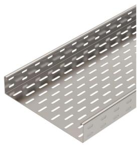
SKS 60 = Heavy-duty cable tray system with 60 mm side height. The cable tray, type SKS, should also be used for maintenance of electrical function. For additional data, please refer to BSS fire protection systems. The cable tray is fastened to the bracket with bolts, type FRS M6 x 12. Magnetic shield insulation without cover 20 dB, with cover 50 dB.
