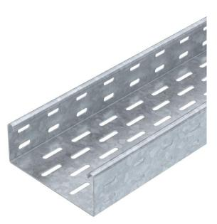
SKS 60 = Heavy-duty cable tray system with 60 mm side height. The cable tray, type SKS, should also be used for the maintenance of electrical function. For additional data, please refer to BSS fire protection systems. Magnetic shield insulation without cover 20 dB, with cover 50 dB.
