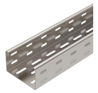
SKS 60 = heavy-duty cable tray system with 60 mm side height. The cable tray, type SKS, should also be used for maintenance of electrical function. For additional data, please refer to BSS fire protection systems. The cable tray is fastened to the bracket with bolts, type FRS M6 x 12.
