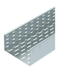
SKS 110 = Heavy-duty cable tray system with 110 mm side height. The cable tray is fastened to the bracket with bolts, type FRS M6 x 12. The surface coating is a coating created in a single-dip method with extra-high zinc thicknesses
