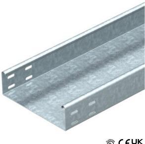
SKS 60 = heavy-duty cable tray system, unperforated, with 60 mm side height. The cable tray has connector perforations on both sides. Straight connectors should be ordered separately and in the appropriate quantity. Magnetic shield insulation without cover 20 dB, with cover 50 dB.
