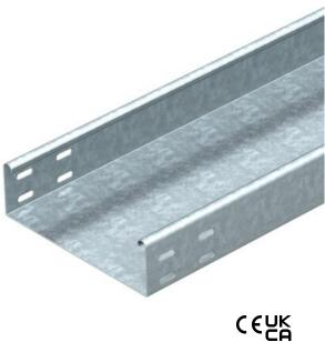
SKS 60 = heavy-duty cable tray system, unperforated, with 60 mm side height. The cable tray has connector perforations on both sides. Straight connectors should be ordered separately and in the appropriate quantity. Magnetic shield insulation without cover 20 dB, with cover 50 dB.
