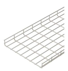
Mesh cable tray made of spot-welded steel wire of side height 55 mm. The grid width is 50 x 100 mm. Magnetic shield insulation without cover 15 dB, with cover 25 dB.
