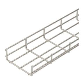
Mesh cable tray made of spot-welded steel wire of side height 55 mm. The grid width is 50 x 100 mm. Magnetic shield insulation without cover 15 dB, with cover 25 dB.
