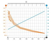
Permitted cable tray/ladder load in kN/m without man load
