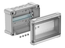
Distribution box for surface mounting, for the current sub-distribution in interior and protected exterior areas, in accordance with IEC 439-3. With pre-mounted 35 mm hat profile rail. IP66 protection type and IK07 protection rating. Transparent cover to screw on, with cut-out.
