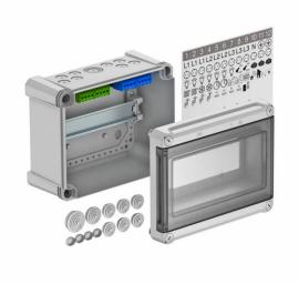
Distribution box with terminal strip for surface mounting, for the current sub-distribution in interior and protected exterior areas, in accordance with IEC 439-3. With pre-mounted 35 mm hat profile rail. IP66 protection type and IK07 protection rating. Transparent cover to screw on, with cut-out.
