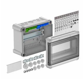
Distribution box with terminal strip for surface mounting, for the current sub-distribution in interior and exterior areas, in accordance with IEC 439-3. With premounted 35 mm hat profile rail. IP66 protection type and IK08 protection rating. Transparent cover to screw on, with cut-out.
