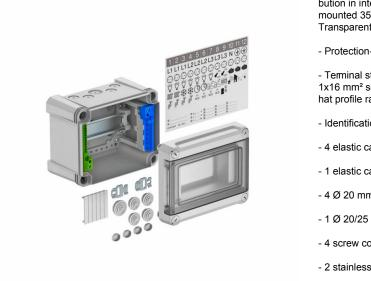
Distribution box with terminal strip for surface mounting, for the current sub-distribution in interior and exterior areas, in accordance with IEC 439-3. With premounted 35 mm hat profile rail. IP66 protection type and IK08 protection rating. Transparent cover to screw on, with cut-out.
