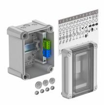
Distribution box with terminal strip for surface mounting, for the current sub-distribution in interior and protected exterior areas, in accordance with IEC 439-3. With pre-mounted 35 mm hat profile rail. IP66 protection type and IK07 protection rating. Transparent cover to screw on, with cut-out.
