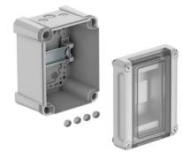
Distribution box for surface mounting, for the current sub-distribution in interior and protected exterior areas, in accordance with IEC 439-3. With pre-mounted 35 mm hat profile rail. IP66 protection type and IK07 protection rating. Transparent cover to screw on, with cut-out.
