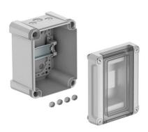
Small distributor for surface mounting, for the current sub-distribution in interior and exterior areas, according to IEC 439-3. With pre-mounted 35 mm hat profile rail. IP66 protection type and IK08 protection rating. Transparent cover to screw on, with cut-out. Including 4 screw cover caps.
