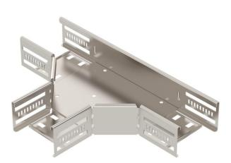
T piece for the creation of a horizontal branch, fitting for lock and screw-on cable trays of side height 60 mm. Screwless mounting with double clamps or screw connection with FRS truss-head screws and M6 combination nuts. Can be used indoors and outdoors. Fastening material must be ordered separately.
